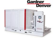
Electra Saver & Electra Saver G2 with infinite positions in an operating range of 40% to 100% capacity, compressor efficiency is maximized because the Turn Valve  $^{\rm IM}$  airend compresses only the volume of air required without affecting the built-in compression ratio at partial load conditions.
